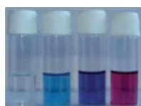
Figure 3. Change in color intensity of 3 ( 5 \times 10^{-5} M) upon the addition of F^- ion (from left to right, free ligand, 1, 2, and 6 equiv) in THF.
